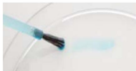
fig. 42: treated surface (72 mN/m)
